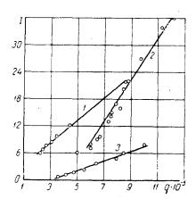
Dependence of acoustic pressure in boiling liquids on heat transfer: 1,2) Water at  $T_0 = 365^\circ$  K and 338° K; 3) alcohol at  $T_0 = 307^\circ$  K. differences  $\Delta T = T_2 - T_1$  at various liquid temperatures. It can be seen from the graphs that at a given temperature of the medium  $T_0$  there is a straight line relation between heat flux and noise intensity.
